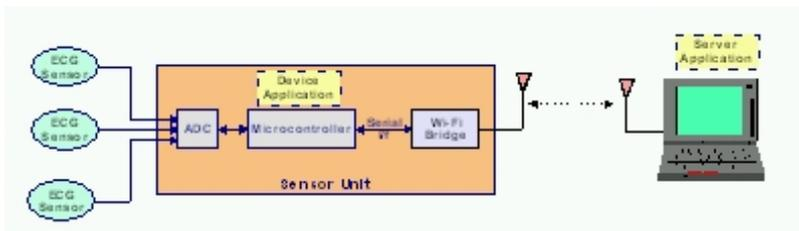
Figure 5: Wireless Connectivity through the Ad-hoc Mode
