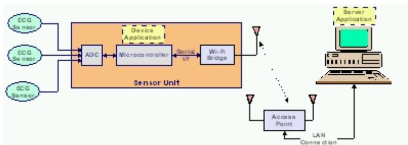
Figure 3: Wireless Connectivity in the Infrastructure Mode
