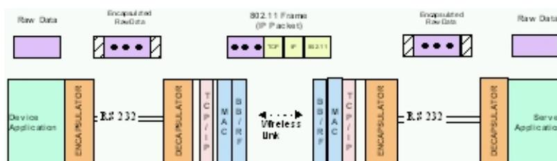
Figure 4: Wireless Connection through a Wi-Fi Bridge
