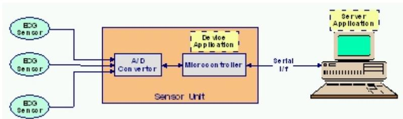
Figure 1: Sensor Unit and Interface to Monitor
