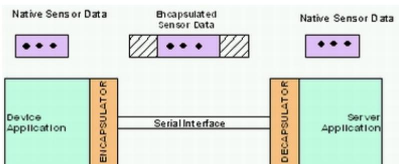
Figure 2: Wired Connection
