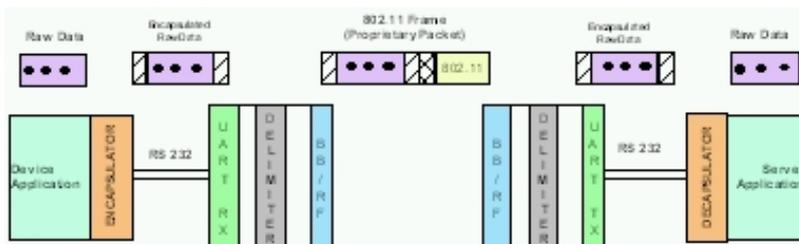
Figure 6: Wireless Transport without TCP/IP
