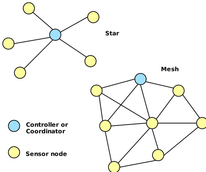
Figure 1: A Wireless Sensor Network
