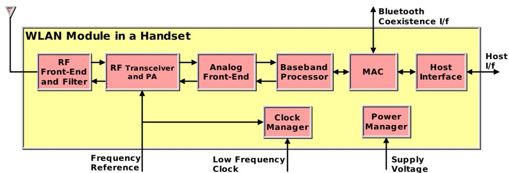
*Figure 1: The Components of a WLAN Module*
