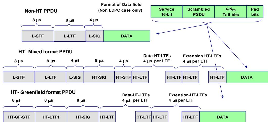
Figure 1: PLCP Frame Structure in 802.11n
