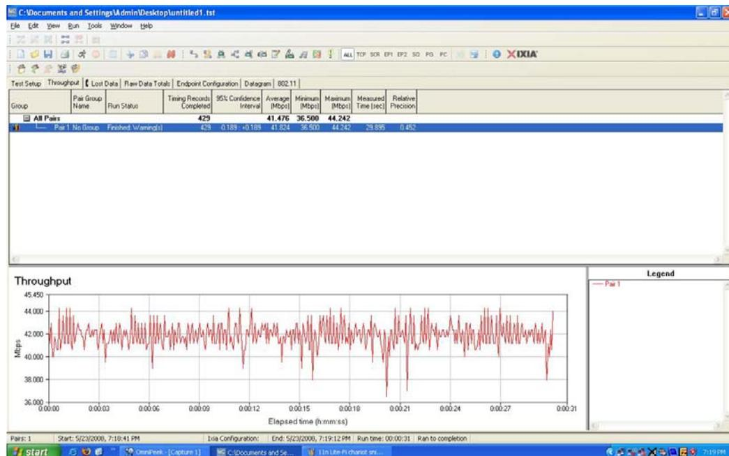
*Figure 8: Throughput in a 11n network in the presence of single stream 1n handheld*
